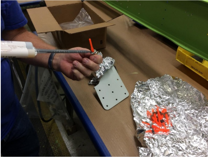
Apply Adhesive 3M Epoxy EC- 3333
