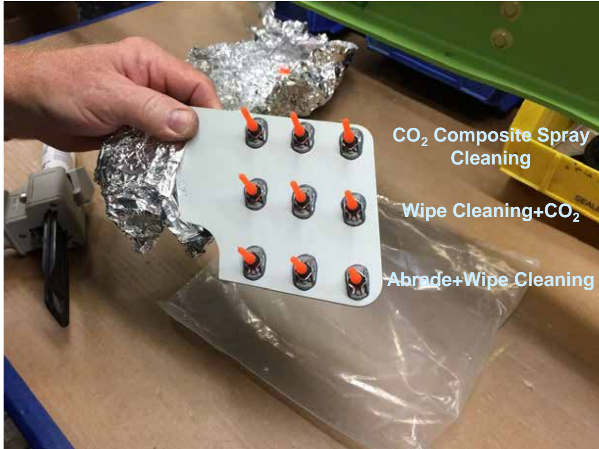
Cured Nutplates (with rubber nutplate tensioners in place)
